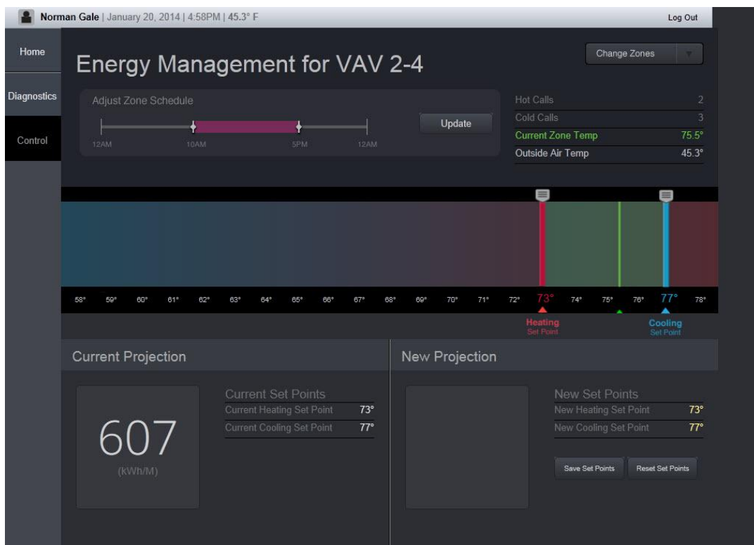
Figure 4: Energy Management and Zone Control Tab
