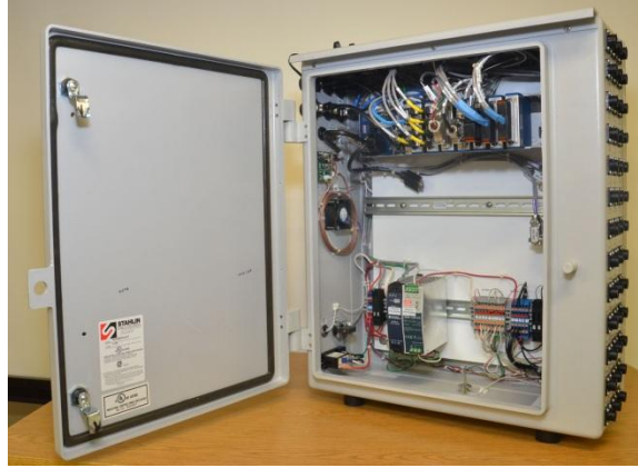
Figure 10 – Completed custom enclosure (note extra room and ports for expansion)
