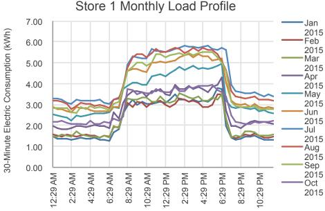
Store 1 shows normal interval data curves, where energy use consistently increases during operating hours. This data shows how summer month electric energy consumption is higher than peak and winter months. Store 1 has case heat service.
