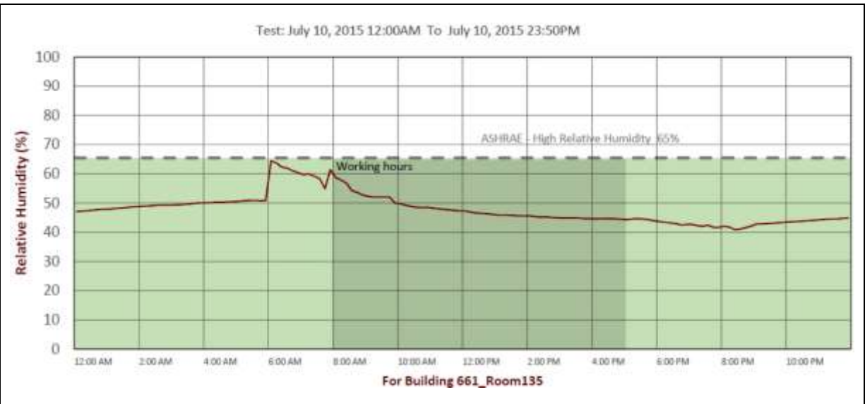
Figure 12 Continuous relative humidity measurements, July 10, 2015(Open office 135)
