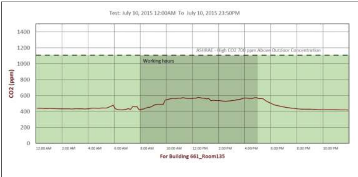
Figure 19 Continuous CO2 Level (ppm) measurements in Open office 135, July 10th
