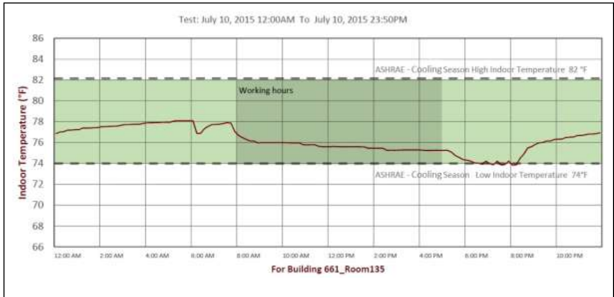
Figure 10 Continuous air temperature measurements , July 10, 2015 (Open office 135)
