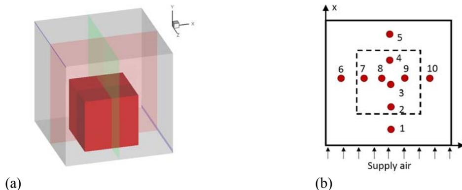
Figure 1 A mixed convection flow in a room (Wang and Chen 2009): (a) the case schematic and the measuring section locations and (b) ten positions selected for comparison between the new model results and the experimental data.
