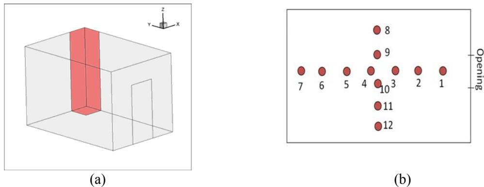
Figure 3 Schematic of the case with strong buoyancy-driven flow (Murakami et al., 1995): (a) the case schematic and the measuring section locations and (b) 12 positions selected for comparison between the new model results and the experimental data.
