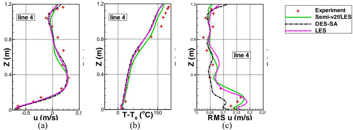
Figure 4 The performance of different turbulence models for: (a) air velocity, (b) air temperature, and (c) RMS velocity.
