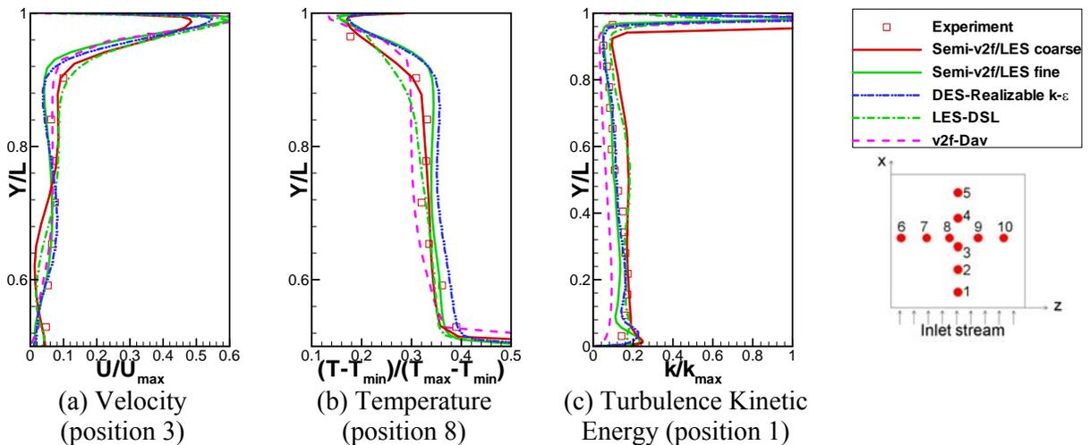
Figure 2 The performance of different turbulence models for: (a) air velocity, (b) air temperature, and (c) turbulence kinetic energy.
