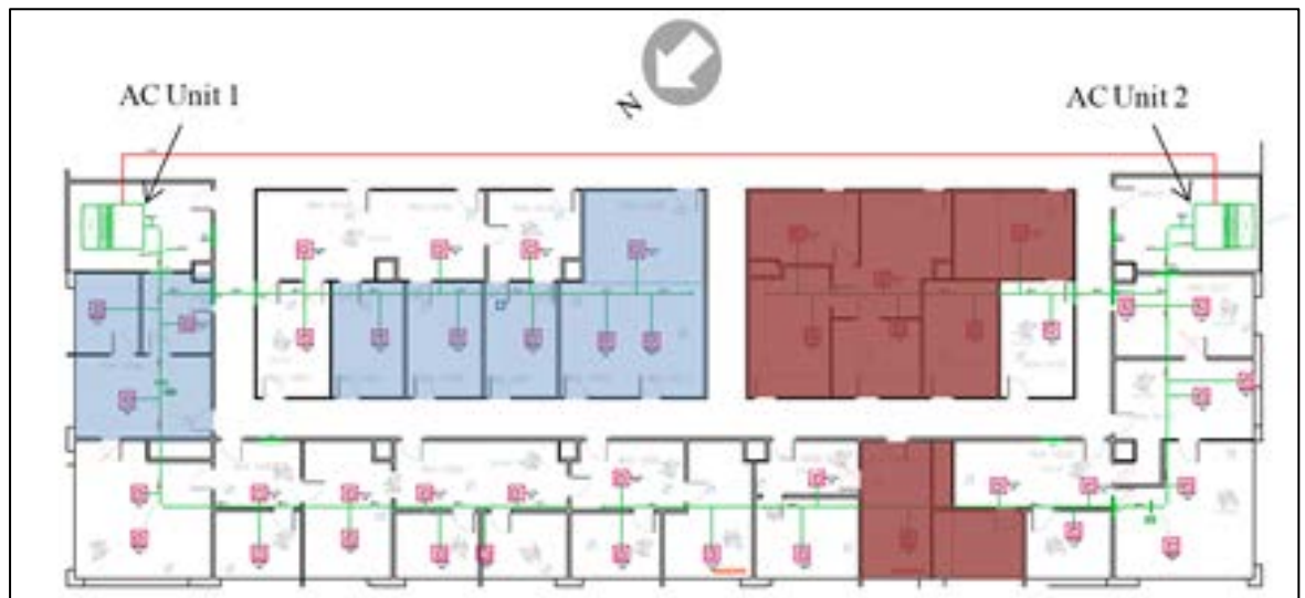
Figure 1 – 4 th Floor West Floor Plan, AHU Location and Duct Layout
