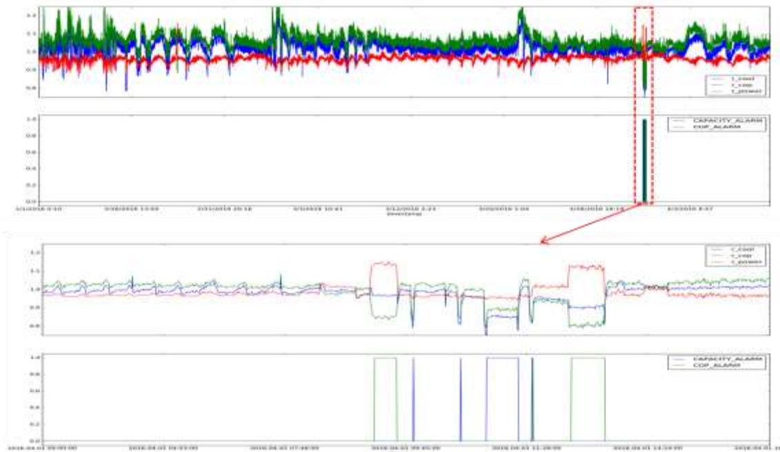
Figure 4.13 Results of AFDD Demo on 2<sup>nd</sup> 7.5 ton RTU (1548 Andalusia Blvd, Cape Coral, FL)
