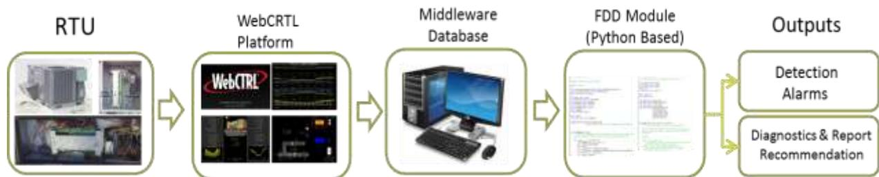
Figure 3.5 Flowchart of Field AFDD Implementation
