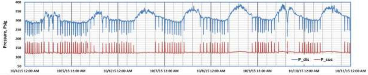
a) 1<sup>st</sup> Stage Compressor Discharge and Suction Pressure
