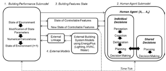
Figure 2: Simulation Modeling Framework (adapted from [7])
