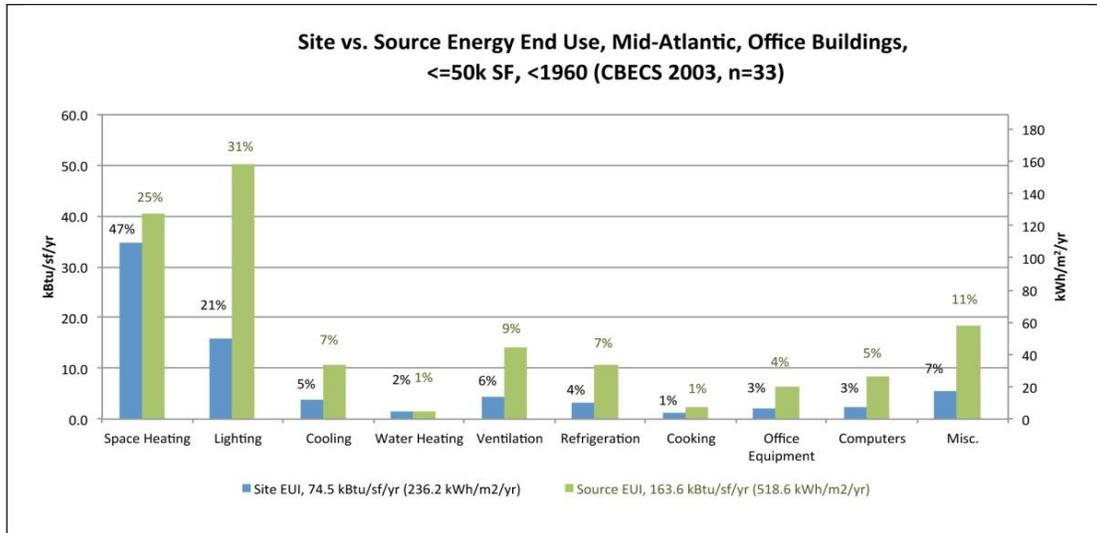
Figure 2 Lighting dominates source energy loads = CO<sub>2</sub> and cost consequences (CBECS, 2003)
