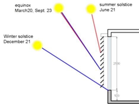
Figure 21 External louver design & sun angles
