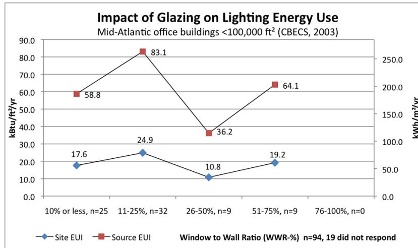
Figure 28 Window area and specification has a significant impact on lighting energy (CBECS, 2003)
