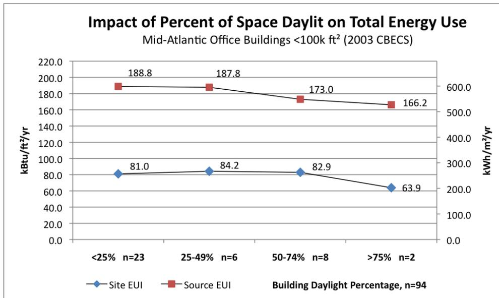
Figure 18 The highest daylight contributions result in the lowest energy use (CBECS , 2003)
