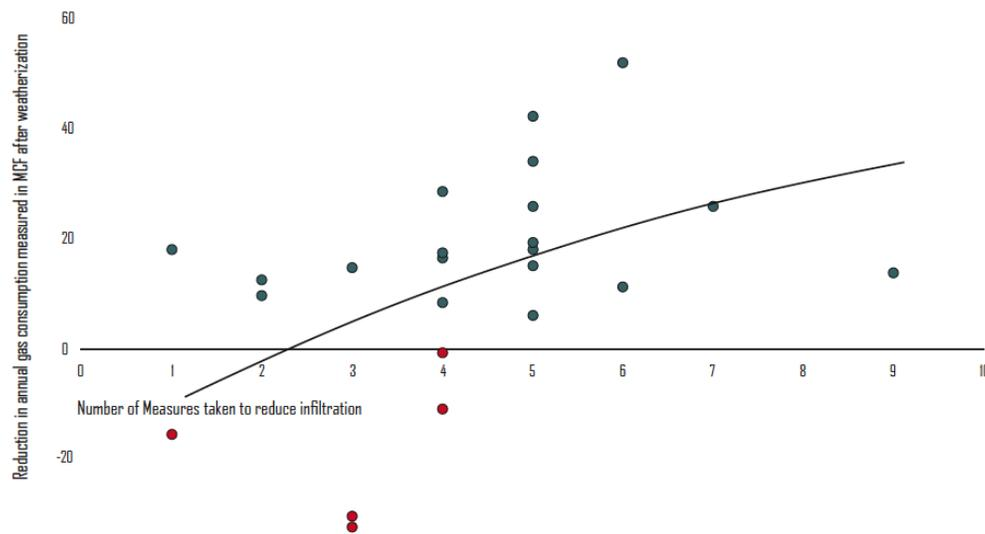
Figure 11 Effect of measures taken to reduce infiltration on annual gas consumption (Tanski, Loftness, Aziz, & Cochran, 2011)
