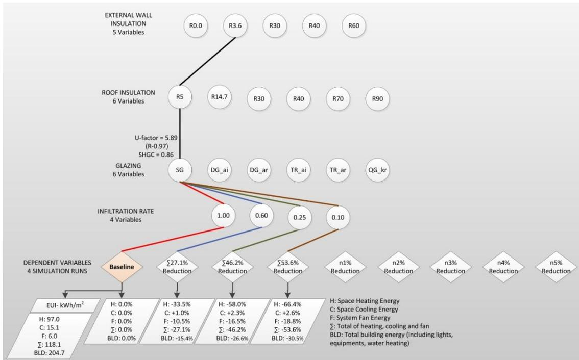
Figure 10 Parametric tree for infiltration rate alternatives (Karaguzel & Lam, 2012)
