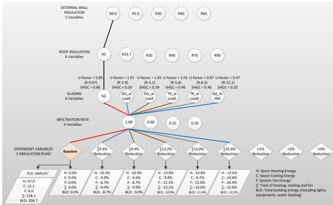
Figure 14 Parametric tree for glazing alternatives (Karaguzel & Lam, 2012)
