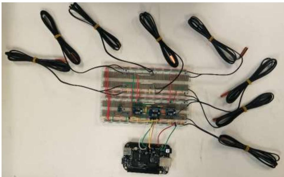
**Figure 2.1. AFDD breadboard prototype hardware including the BeagleBone Black development platform and thermistor temperature sensors.**
